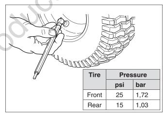
Figure 14. Checking Tire Pressure
